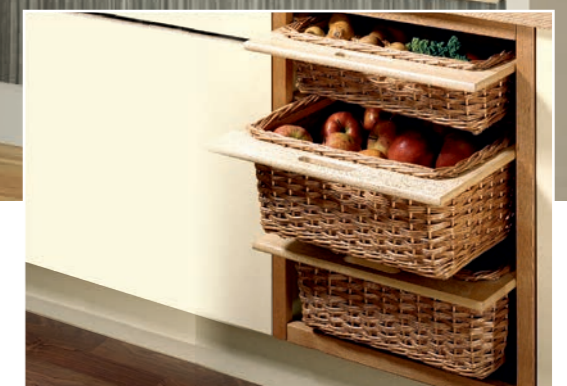
3. Wicker basket ▶ With wooden frame and integrated handle moulding. ▶ For cabinet widths of 400, 500 and 600 mm, minimum carcass depth inside 500 mm. ▶ With roll-out prevention. ▶ Wooden frame solid beech.
