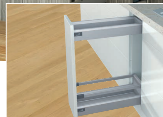
2. Narrow base unit ▶ Carcase height 750 mm max. ▶ Carcase width 300 mm max. ▶ Actro drawer runner is required on the left and right, mounted diagonally.
